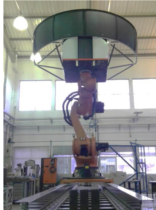
Fig. 10. The high fidelity SIVOR flight simulator.
