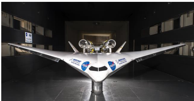
Figure 7. BWB model with ejectors nacelles in 14x22 tunnel
