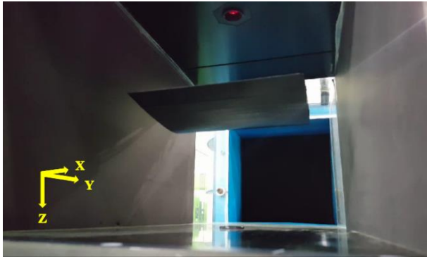
Fig. 6. Magnetic Levitation of the Finite Wing Model
