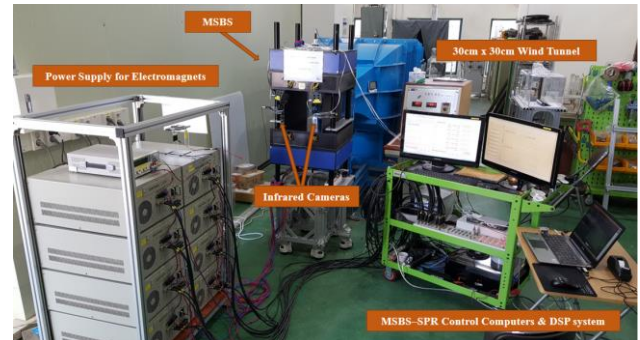
Fig. 7. KAIST MSBS Installed at Wind Tunnel [10]
