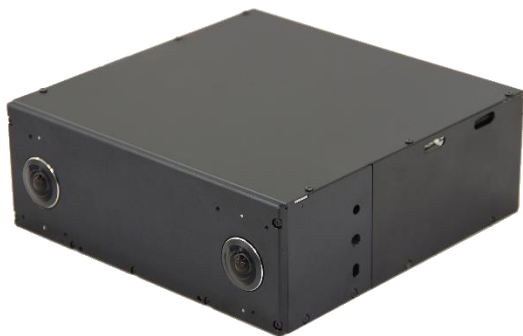
Fig. 2 Super wide angle stereo vision system
