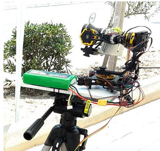
Figure 3. Setup for ground testing of EO camera module
