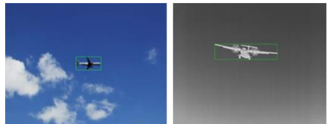
Figure 11. Aircraft detected by EO camera module (left) and IR camera module (right)
