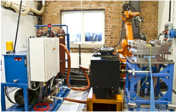
Fig. 2. Varestraint test equipment.
