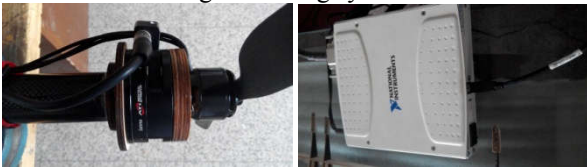
Fig 13 Six-component balance (left) and data collector (right)
