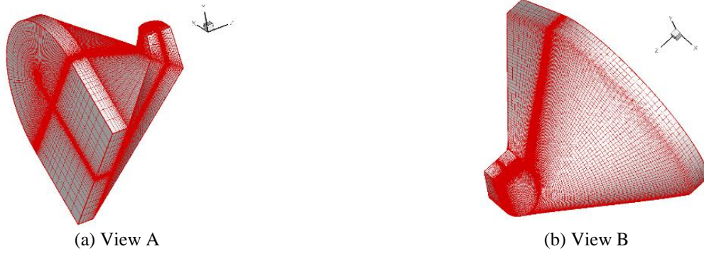
Fig. 2 Schematic of the grid for the propeller with the proplet
