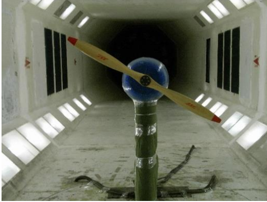
Fig. 7 Propeller model with 1.2m diameter(NF-3 wind tunnel of Northwestern Polytechnical University)
