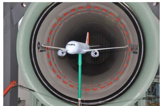
Fig. 1. The photo of force measurement test
