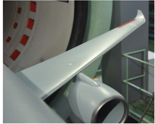
Fig. 4. Photos of the severe ice shape on the wing
