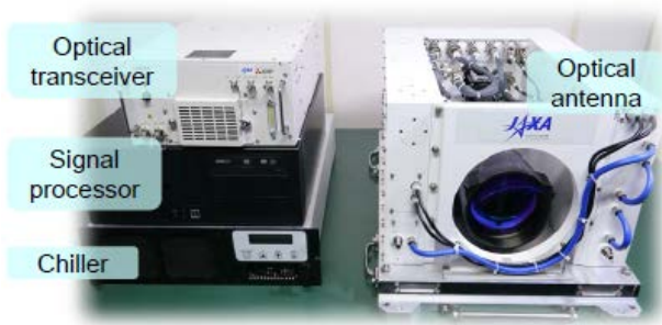
Fig. 1. Developed Doppler LIDAR wind sensor.
