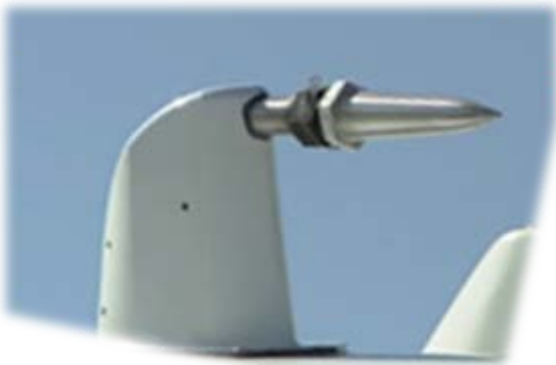
Fig. 3. Inlet Probe Mounted on the Aircraft.
