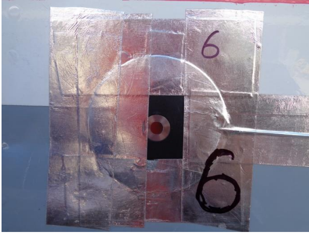
Fig. 2 Microphone Mounting on the Fuselage
