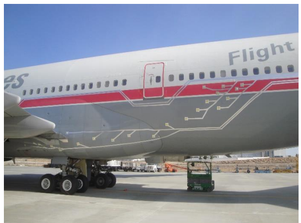
Fig. 5 Surface microphones on the aft fuselage
