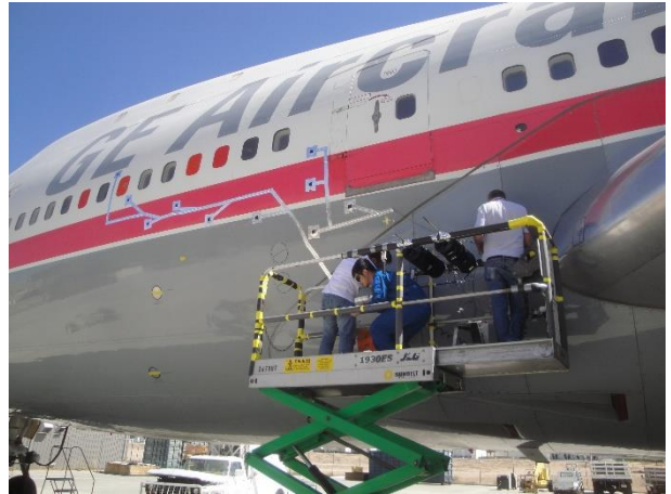
Fig. 4 Install microphones on a lift platform
