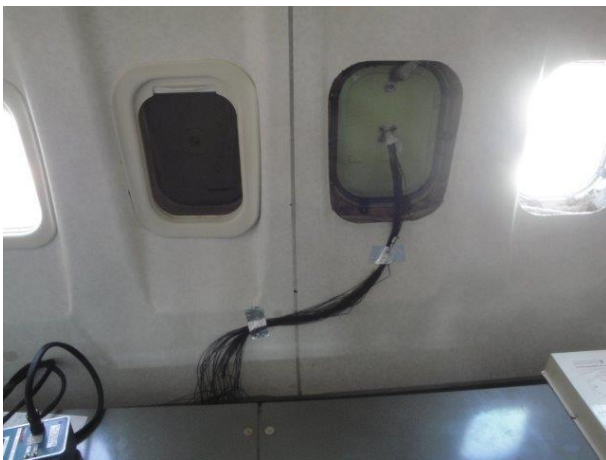
Fig. 3 Cables passing through the dummy window
