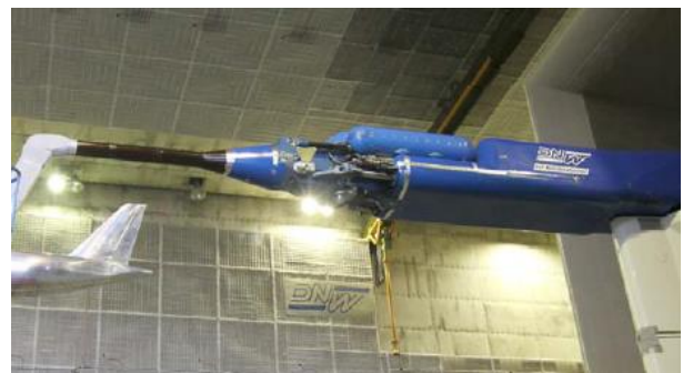
Fig. 3 Sting without fairing, configuration with vertical tail
