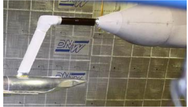
Fig. 2 “New” fairing, configuration without vertical tail showing dorsal (left) and sting
