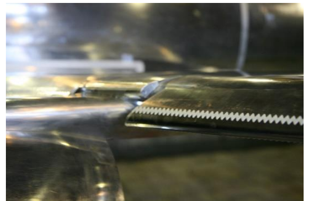
Fig. 14 Zig-zag tape applied on the slat upper and lower (not shown) surface of the slat
