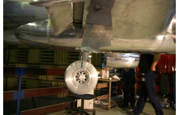
Fig. 17 Details of the wheel showing the holes responsible for the whistle noise at 3.5 kHz Config. B - 70m/s
