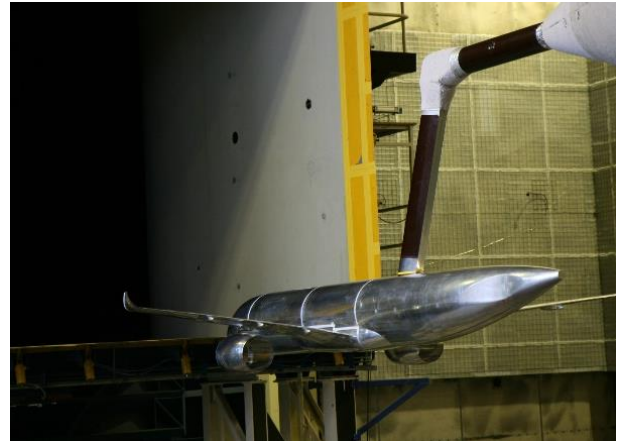
Fig. 6 Aircraft model position below the shear layer of the open jet, and dorsal sting exposed to the flow, configuration A3
