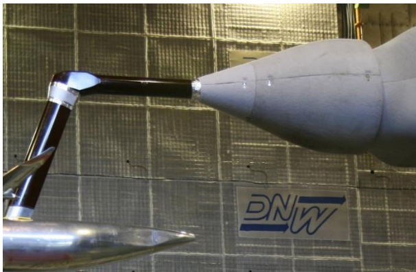
Fig. 5 Same as figure 3 but without the acoustic treatment around the dorsal sting.
