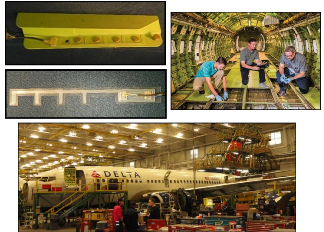
Fig. 5. Long-term flight testing of CVM sensors on operating aircraft
