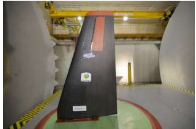
Fig. 4. The semi-span wing model in the wind tunnel T-3
