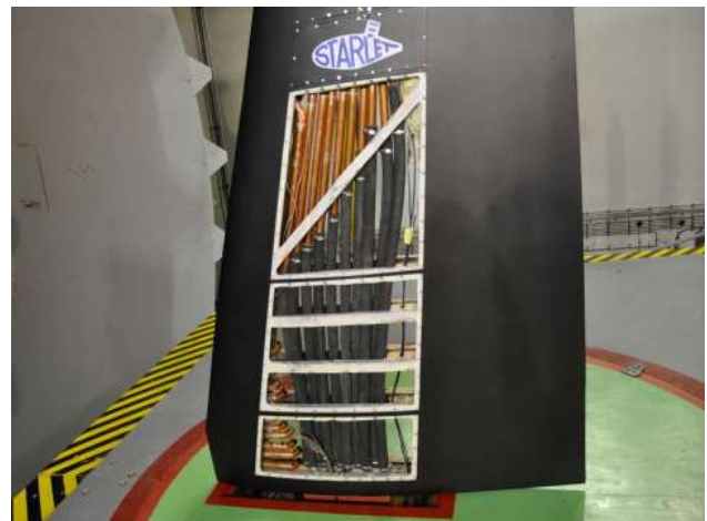
Fig. 5. The system of pipes supplying active load control devices with air
