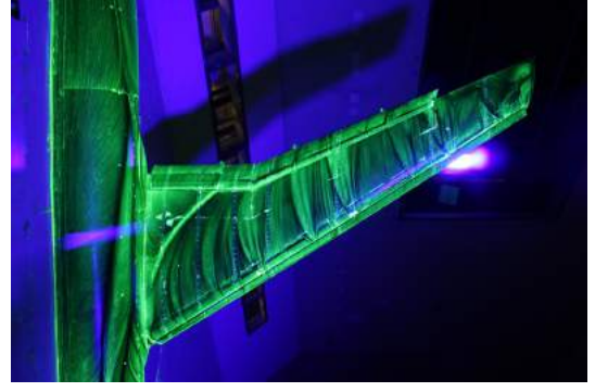
(a) Experimental data: Oil flow visualization
