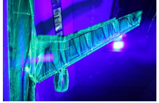
(a) Experimental data: Oil flow visualization
