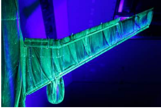
(a) Experimental data: Oil flow visualization
