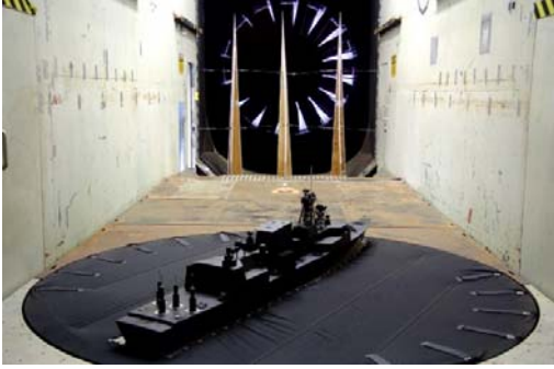
Figure 9. Setup of the oscillating CPF model in the wind tunnel.
