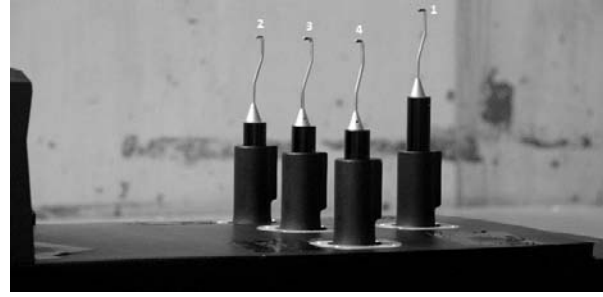
Figure 10. An array of Cobra probes mounted on the flight deck of the oscillating CPF model.
