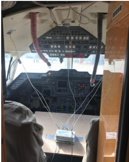
Fig. 6. Location of the Thermocouples inside the Hawker 800 aircraft. (Own authorship)
