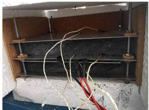
Fig. 4. Location of the Thermocouples on the Specimen. (Own authorship)
