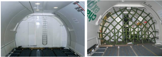
Figure 24: B737Classic/NG 9g Rigid Barrier and 9g Safety Net
