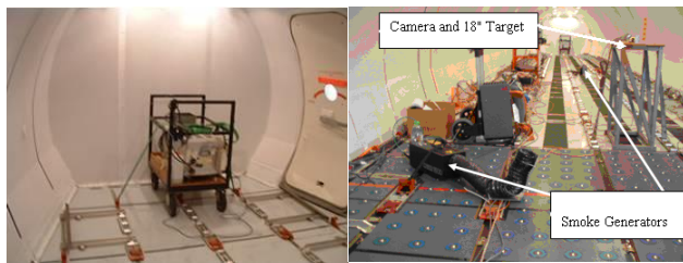
Figure 18: B737NG Smoke Detection and Penetration Ground & Flight Tests
