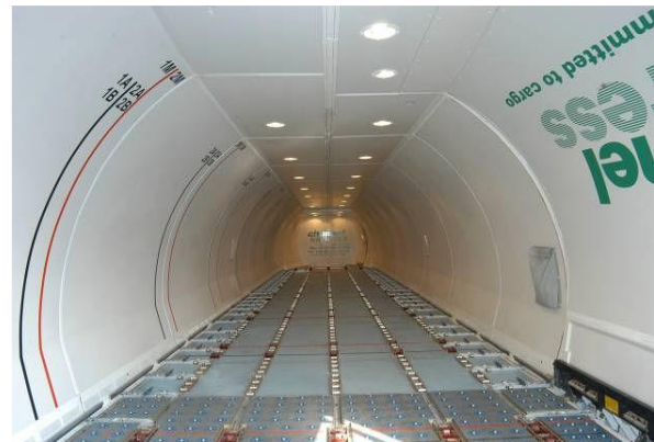
Figure 22: B737NG Cargo Loading System
