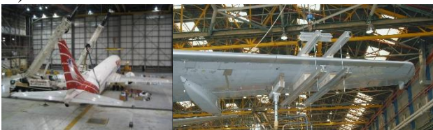
Figure 10: B737 Center of Gravity and Ground Vibration Test (GVT) Evaluation
