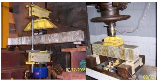
Figure 25: 9g Barrier Shear & Bending Tests
