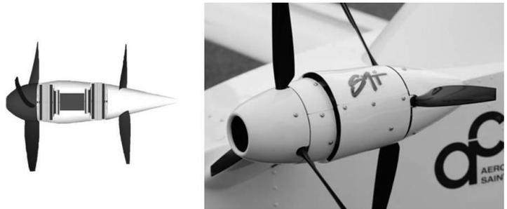
Figure 1: Electric motors configuration and air inlets visualization
