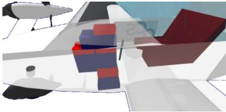
Figure 4: Battery Pack integration
