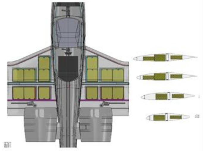
Figure 6: Battery Installation
