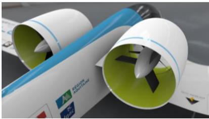
Figure 5: Electrical Ducted Fan
