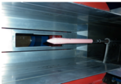
Fig. 6. Model painted with PSP and installed in the TTP test section.
