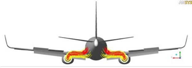
Fig. 11. Back view of existing jets from exhaust nozzle (red) and bypass duct (yellow).
