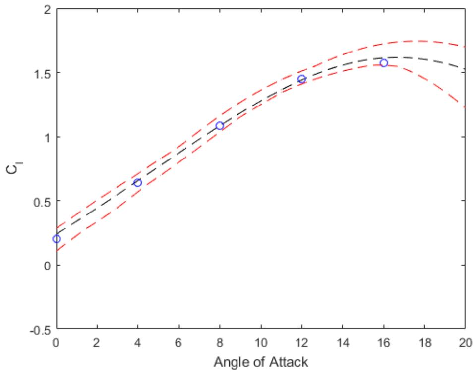
**Fig. 3** Lift coefficient predictions of a NACA 2410 airfoil as a function of angle of attack.
