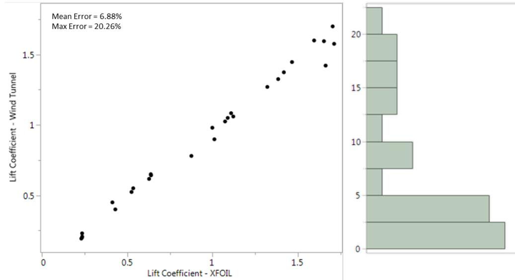
**Fig. 2** Plot of the actual lift coefficient from the wind tunnel data versus the predicted lift coefficient from XFOIL. A histogram of the error is shown to the right of the plot.
