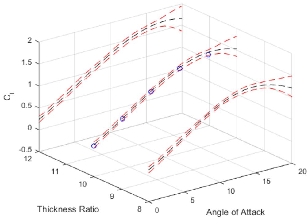
**Fig. 4** Lift coefficient predictions of a NACA 24XX airfoils as a function of angle of attack and thickness.
