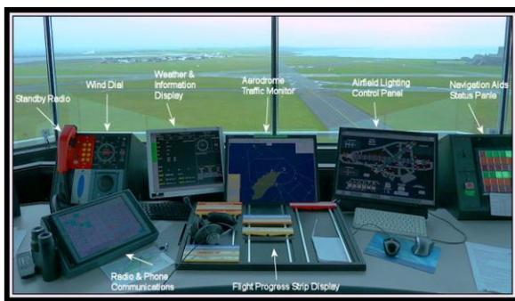
**Fig. 5. ATCO workstation at a relatively small airport** (Ronaldsway Airport, Island of Man , photo: Jon Wornham - <http://www.island-images.co.uk/ATC/zRon2014/1009221616.html>)
