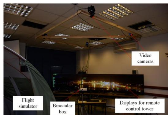
Fig. 8. The investigated eye tracking system control system
