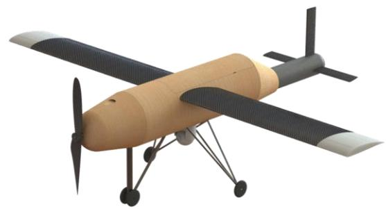
Fig. 8. 2014-15 Team 1 final design of an affordable, rapid response UAV to meet RFP requirements
