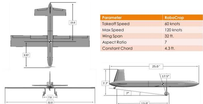
Fig. 11. 2015-16 design team final design of an AUAS to meet RFP requirements
