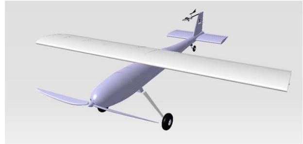
Fig. 4. 2013-14 Team 1 final design of a search and rescue UAV to meet RFP needs
