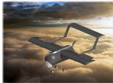
Fig. 5. 2013-14 Team 2 final design of a search and rescue UAV to meet RFP needs
