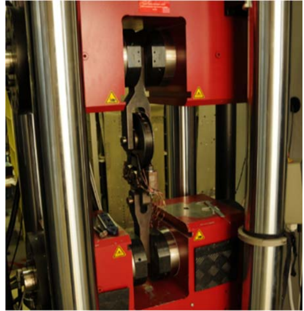
Fig. 15. Metal-Composite Joint in Testing Machine.
