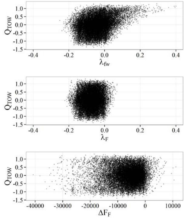
Fig. 8. Weight quotient  $Q_{TOW}$  over  $\lambda_{fw}$ ,  $\lambda_F$  and  $\Delta F_F$  for the *complete set* and all formation pairings
