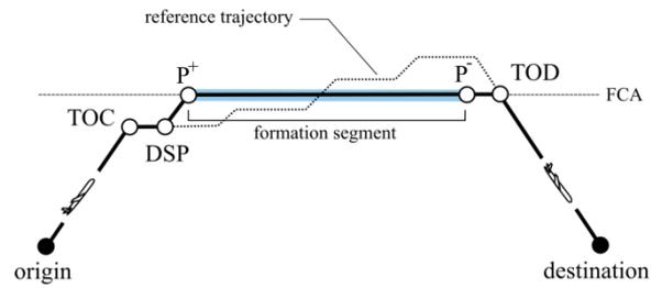
Fig. 2. Typical vertical flight profile of a formation member
