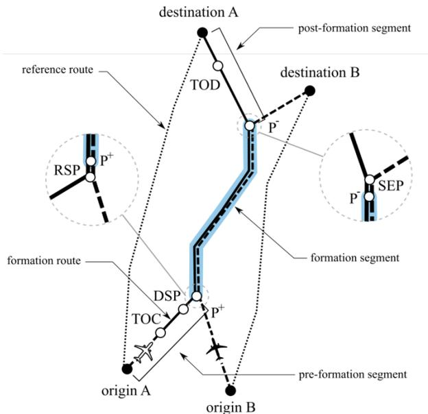
Fig. 1 Schematic lateral formation geometry of a two-aircraft formation
