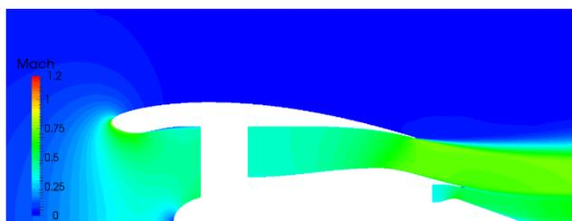
Fig. 6. Nacelle optimal geometry, Mach number field at takeoff regime  $M_\infty = 0$
