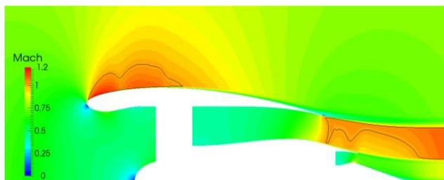
Fig. 5. Nacelle optimal geometry, Mach number field at cruise regime  $M_\infty = 0.78$
