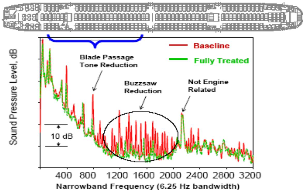
Fig.5. Spectrum interior noise (forward cabin) aircraft-demonstrator QTD2 [7].
