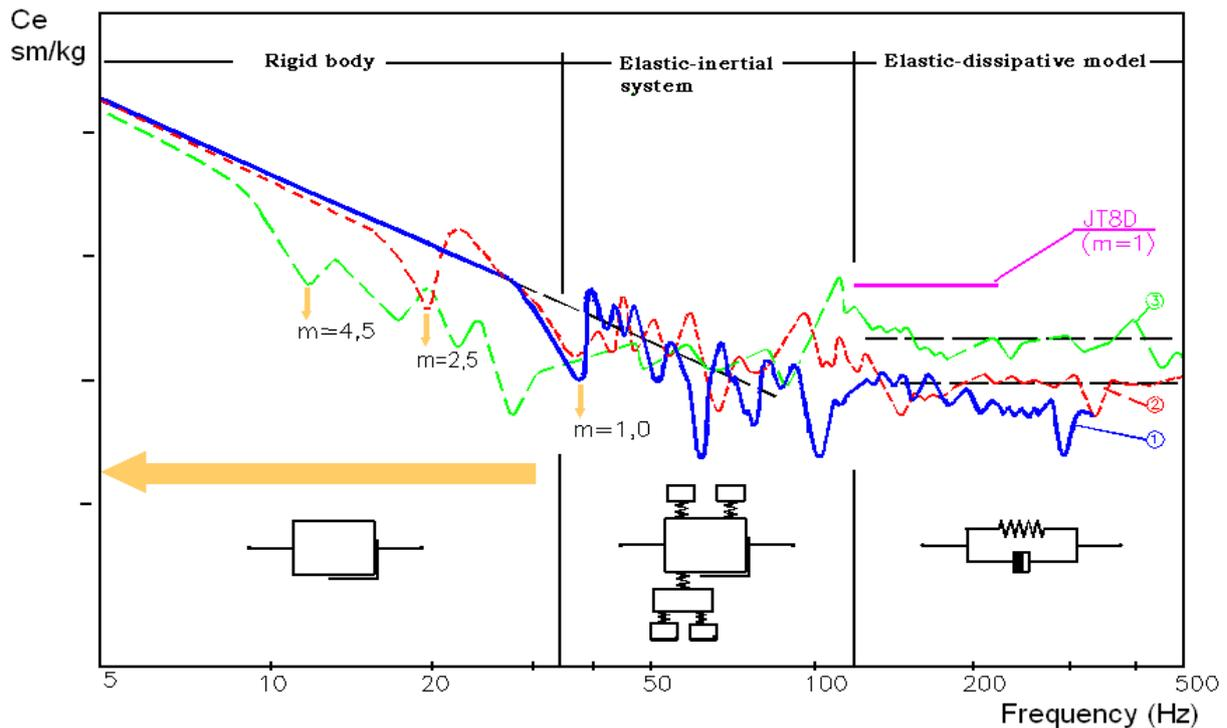
Fig.2. Dynamic compliances of engine body at attachment points
