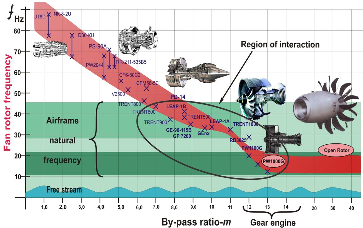
Fig.4. Change of frequency of fan shaft rotation at degree increase by-pass ratio of engines.
