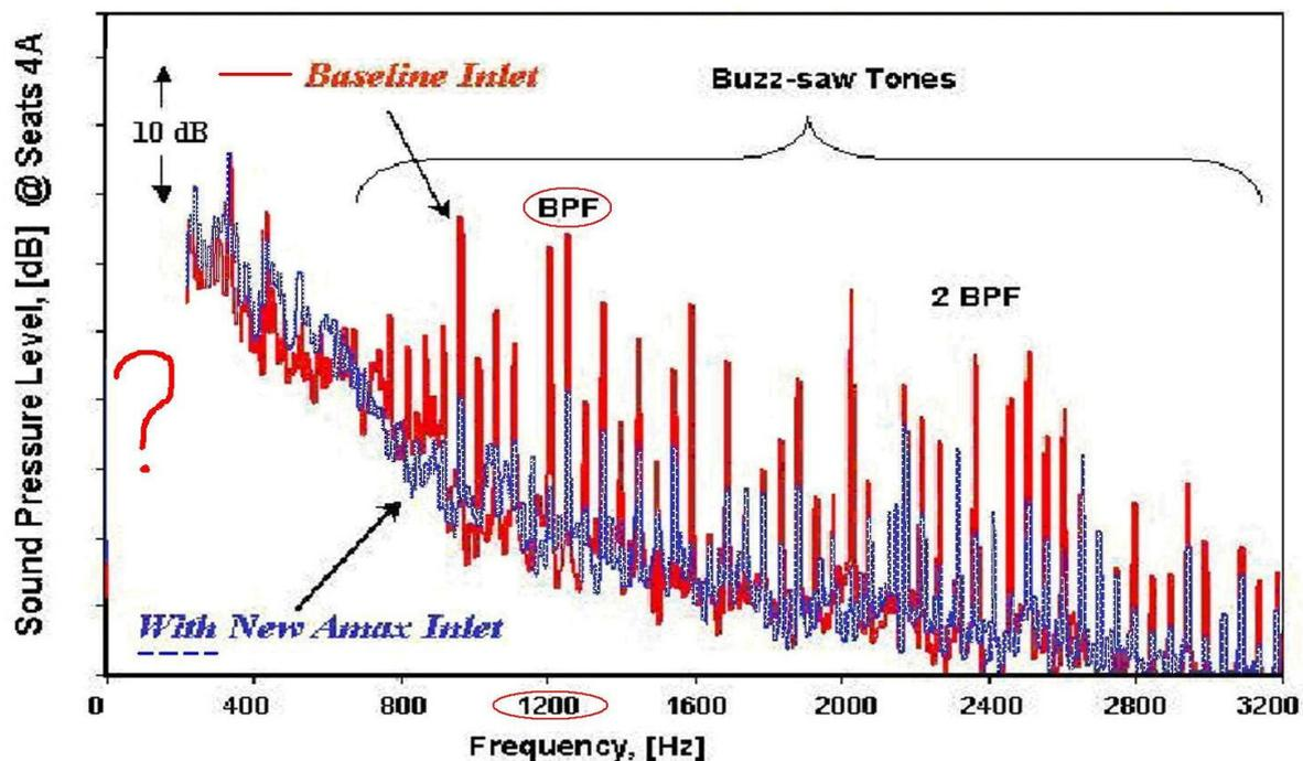
Fig.3. Spectrum interior noise of forward cabin aircraft-demonstrator QTD1
