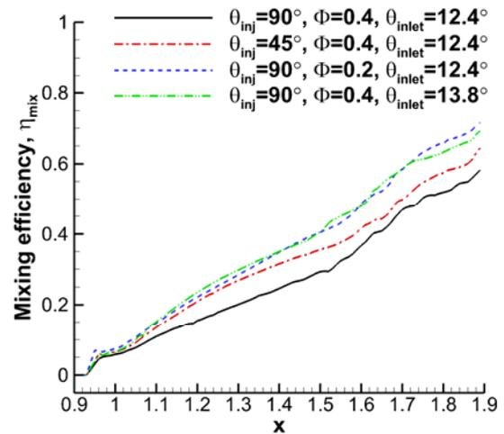
Fig. 5. Mixing Efficiency Comparison for Varying Injection Angle, Equivalence Ratio and Inlet Ramp Angle.
