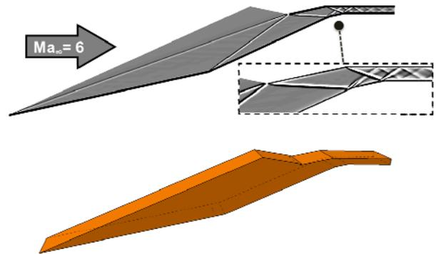
Fig. 2. Two-dimensional Shock Pattern (top) and Three-dimensional Geometry (bottom) of Inlet.
