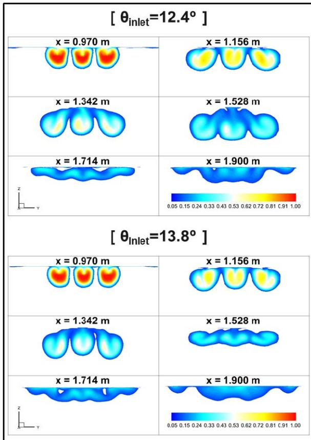
**Fig. 8. Comparison of Ethylene Mass Fraction Contours between Different Inlet Ramp Angles.**
