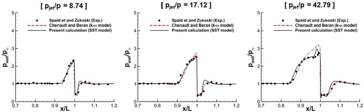
Fig. 1. Comparison of Surface Static Pressure Distributions for Spaid and Zukoski's Configuration [12].
