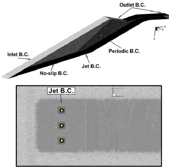
Fig. 3. Computational Domain and Boundary Conditions.
