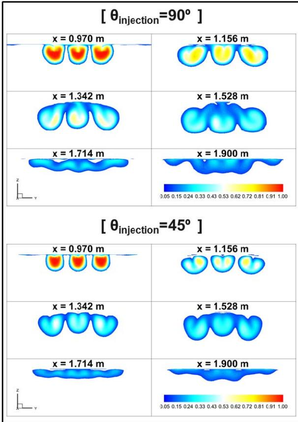
**Fig. 6. Comparison of Ethylene Mass Fraction Contours between Different Injection Angles.**
