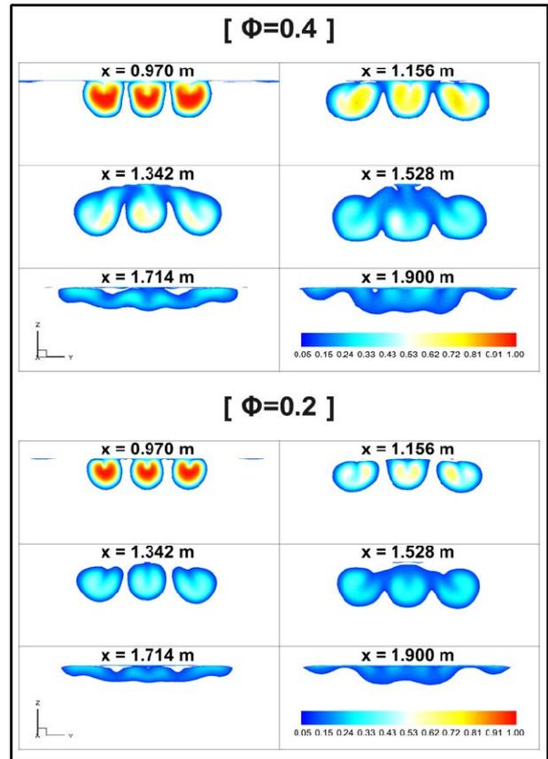
**Fig. 7. Comparison of Ethylene Mass Fraction Contours between Different Equivalence Ratios.**
