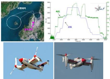
Fig.1. Flight Trajectory and Speed & Altitude of Smart UAS Flight Test (One hour Flight with Max. Speed of 440km/h at 3km Alt.)
