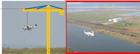
Fig.14. Tethering and Free Flight Tests of 40% Small scaled Flight Demonstrator
