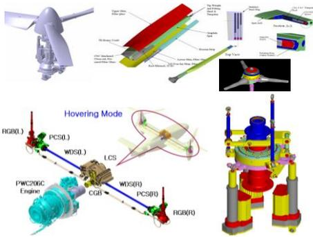
Fig.9. Prop-Rotor System Design
