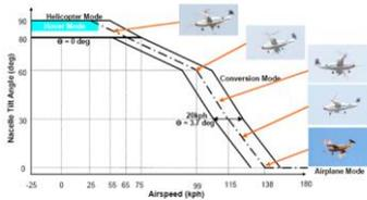
Fig.15. Conversion Corridor of 40% Small scaled Flight Demonstrator
