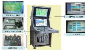
Fig.11. Ground Control System
