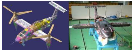
Fig.8. FEM Model and Static Structural Test
