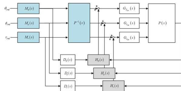
Fig. 2. Model Following Control(MFC) system
