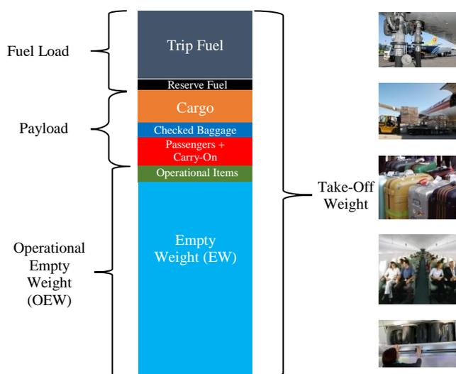
Fig. 1: Aircraft take-off weight breakdown.
