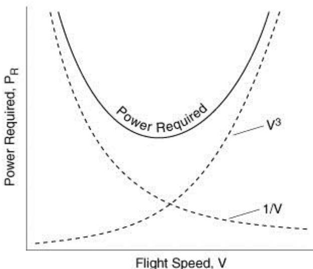
Fig. 7: Typical Airplane Power Curve
