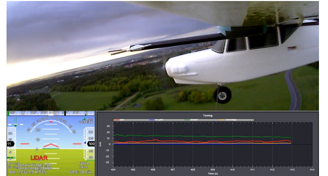
Fig. 11 . Evaluation of the small AOA transducer performance and calibration by comparing logged flight data with visual references captured by a micro-camera.
