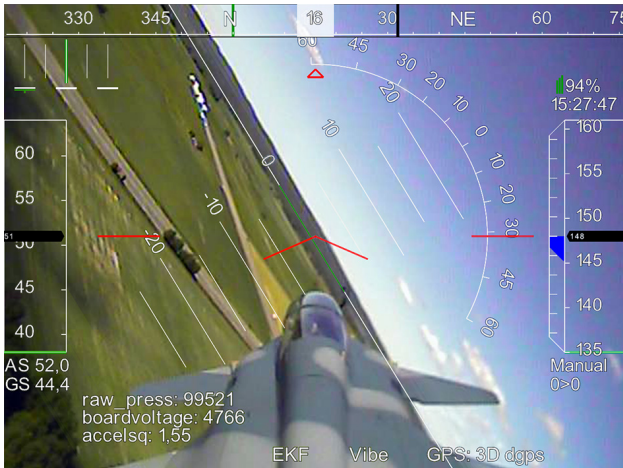
Fig. 13 . One of the jet-powered platforms performing sustained high-g turns to test the robustness of the attitude estimation. Flight data are superimposed on real video using the open-source software Mission Planner [26].
