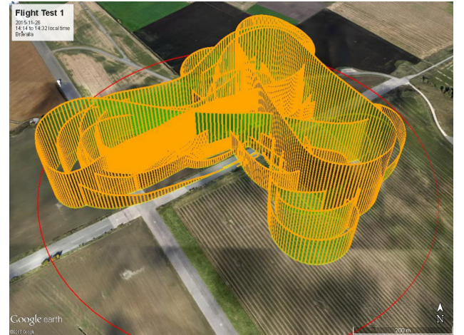
Fig. 16 . Trajectory reconstruction of a flight test exported into Google Earth using the open-source software Mission Planner [26].
