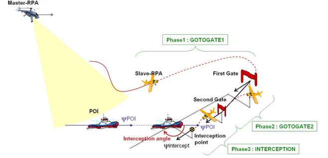
**Fig. 5** Three-step target interception guidance procedure
