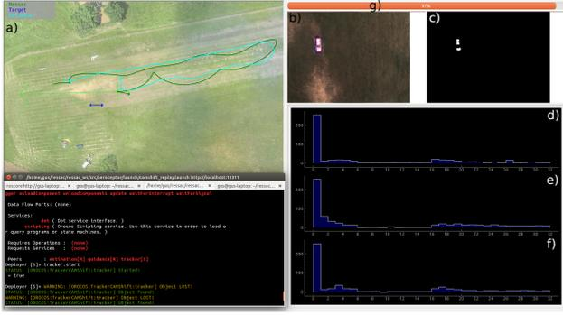
**Fig. 3** a) Local map with RPA and POI trajectories, b) Raw images with detected objectBox and boundingBox, c) Back projection of the image using the POI histogram, d) POI's reference histogram, e) POI histogram, f) Full image histogram, g) Confidence level.
