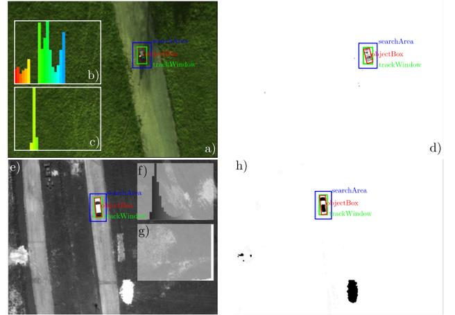
**Fig. 2** a,e) Original RGB/grayscaled image with the tracking results, b,f) POI's histogram, c,g) The background histogram, d,h) The back projection and results of the CAMSHIFT algorithm.
