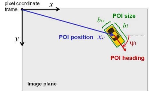
**Fig. 4** Vision-based measurements for POI localization
