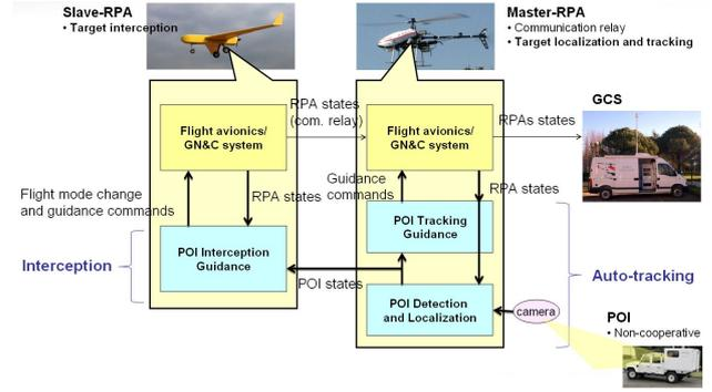
Fig. 1 Onboard systems on the Master- and the Slave-RPAs
