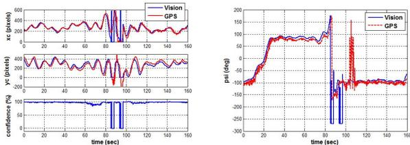
Fig. 9 Vision-based measurements: (left) pixel coordinates and confidence level, (right) heading angle
