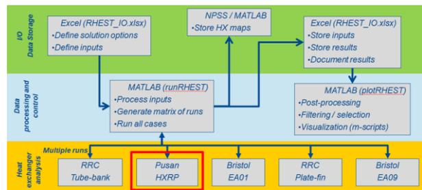
Figure 9, RHEST interfaces and data flow.
