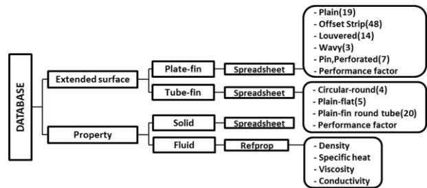
Figure 8, Structure of the heat exchanger database
