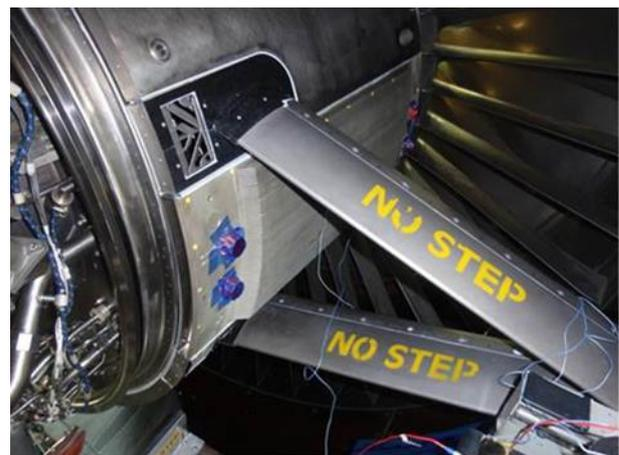
Figure 5, SHAFAE panel type heat exchanger
