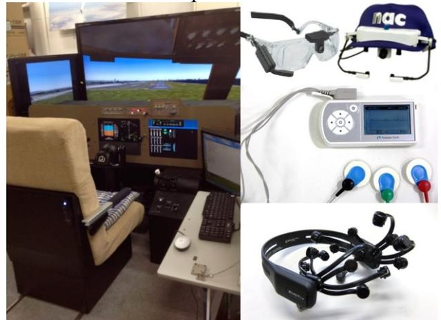
Fig. 5 Boeing 747-400 simulator at the University of Tokyo and the Takei TalkEyeLite and NAC EMR8 eye-mark cameras, ParamaTech EP-301 portable ECG recorder, and eMotiv EPOC+ eeg headset..
