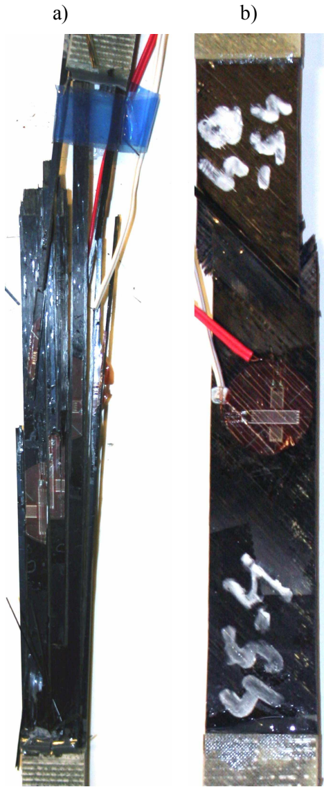
Fig. 7. Typical failure modes for the CFRP test specimens: (a) UD specimen; (b) shear specimen.
