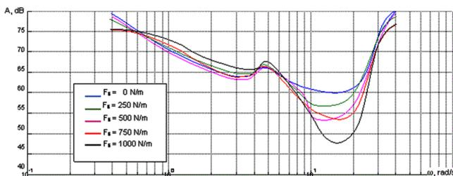
Fig. 5. Averaged frequency responses of neuromuscular system for different force gradients (sidestick).
