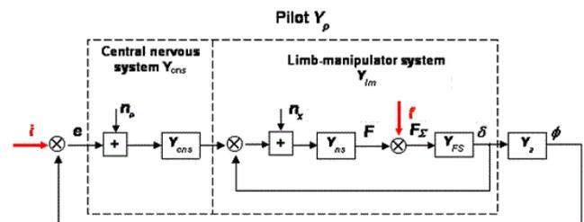
Fig. 2. Structure of pilot model in roll tracking task.
