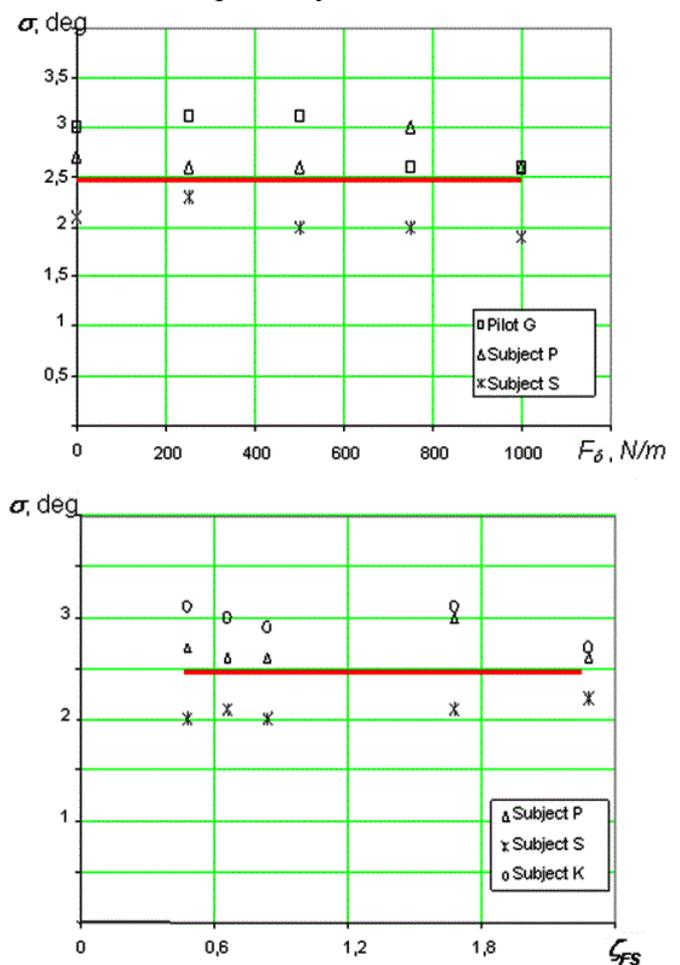
Fig. 1. Tracking accuracy as a function of manipulator force gradient ( $F_{\delta}$ ) and damping ratio ( $\zeta_{FS}$ ).
