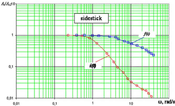
Fig. 3. Visual  $i(t)$  and force  $f(t)$  forcing functions used in roll tracking task with wheel (upper picture) and sidestick (lower picture).
