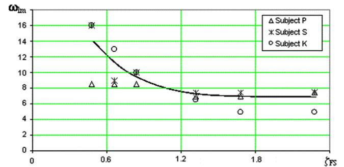
Fig. 10. Cutoff frequency of the limb-manipulator open-loop system as a function of damping ratio for a sidestick ( $F\delta=500$  N/m).
