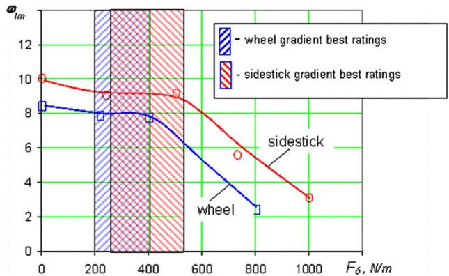
Fig. 9. Cutoff frequency of the limb-manipulator open-loop system as a function of force gradients for the wheel and sidestick.
