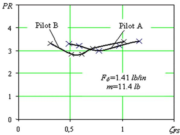
Fig. 7. Pilot ratings as a function of damping ratio (wheel, roll axis).
