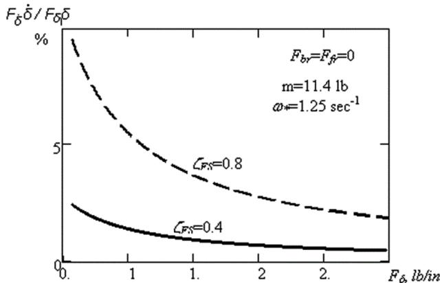
Fig. 8. Damping contribution to the total manipulator force (wheel, roll axis).
