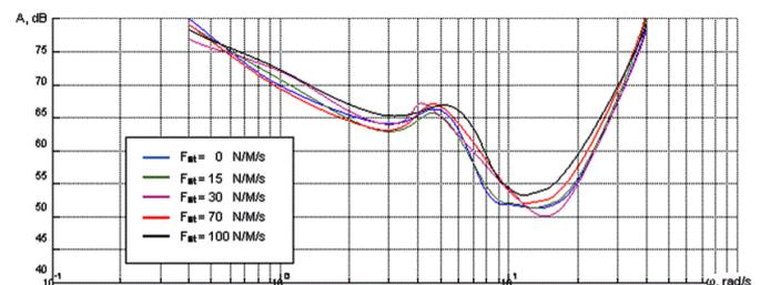
Fig. 6. Averaged frequency responses of neuromuscular system for different damping (sidestick).
