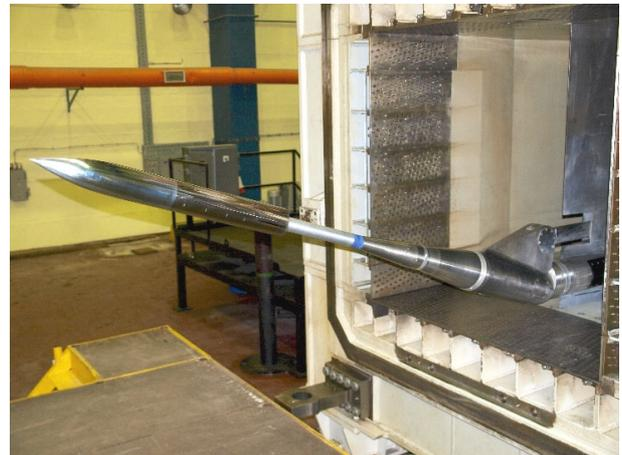
Fig. 6. The 115.8 mm dia. with 0.53% blockage AGARD-B model in the T-38 wind-tunnel
