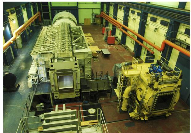
**Fig. 1.** The T-38 wind tunnel opened with transonic test section to be installed in tandem within the circuit
