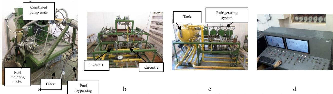
a – combined pump (gear stage and screw-centrifugal stage), hydromechanical fuel metering unite, fuel aggregates; b – a system for combustion chamber simulation; c – fuel supply system and refrigerating system; d – operator station
