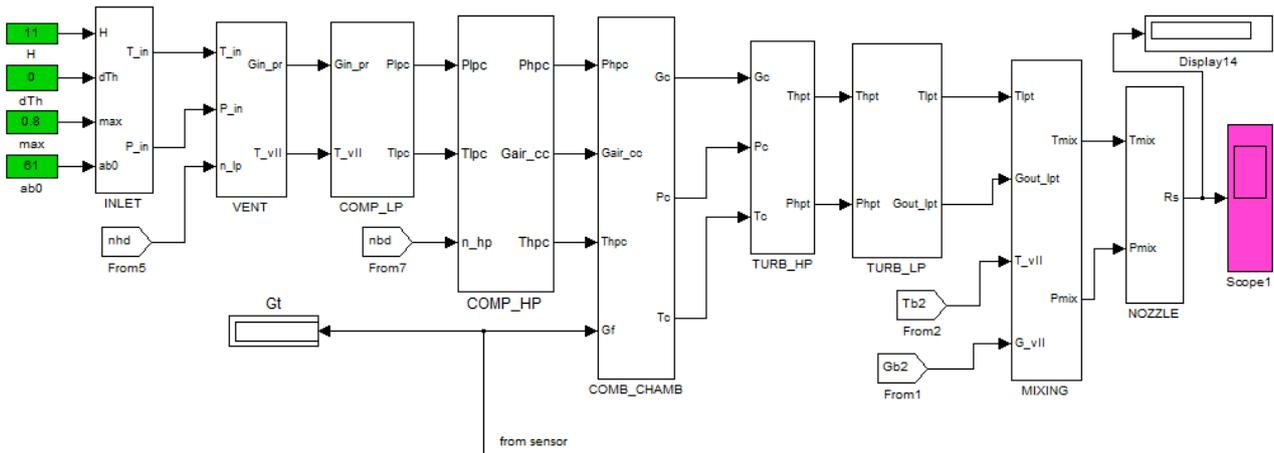
‘Fig. 3. The Subassembly Mathematical Model of Turbofan Engine (MATLAB Simulink)’
