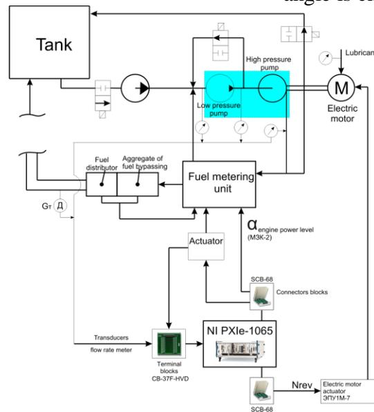
'Fig. 2. The Circuit Diagram of the SSAU HIL Bench'
