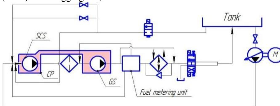
SCS – screw centrifugal stage; CP – centrifugal pump; GS – gear stage
