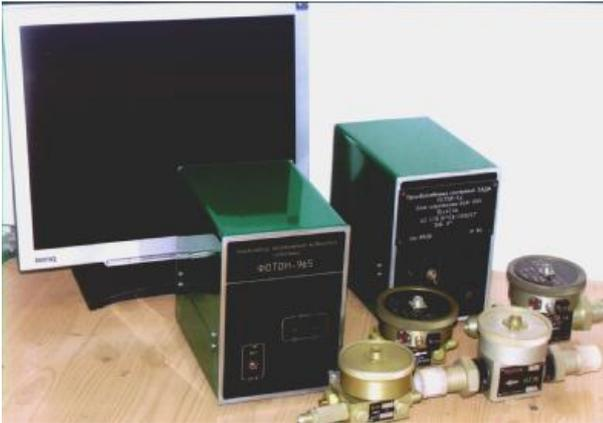
Fig. 3. Integrated sensor of fluid contamination control
