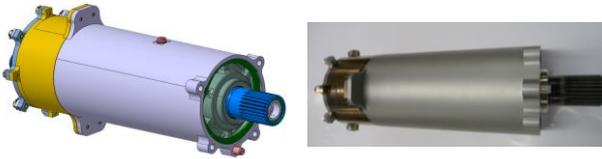
**Fig. 4: FRACASS Rotary EMA [18]**
