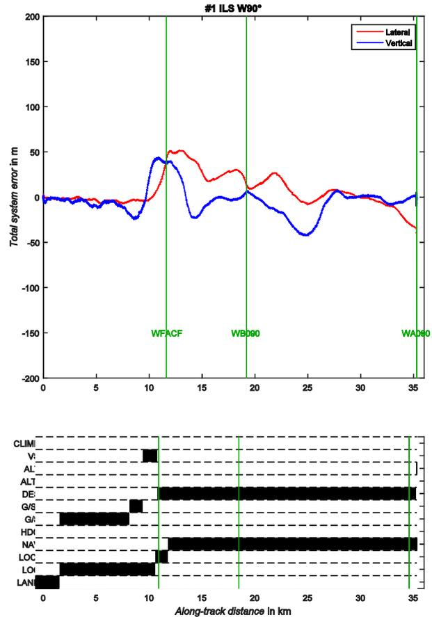
**Figure 3 ILS W90 from 16 July 2015. The top panel shows lateral and vertical flight technical error, the bottom panel indicates autopilot modes active during the approach. Green lines mark the approach waypoints. The aircraft arrived slightly high at WFACF which was corrected by the pilot using VS mode**
