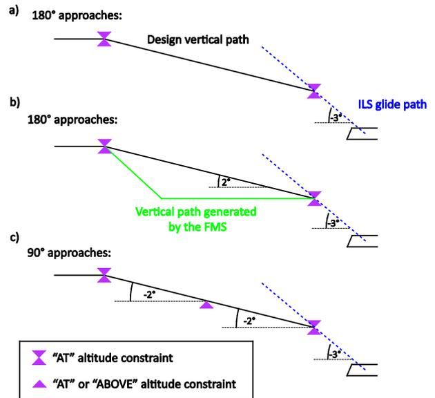
Figure 2 Vertical path coding with and without flight path angle. Design vertical path and „dive and drive” behavior of the aircraft
