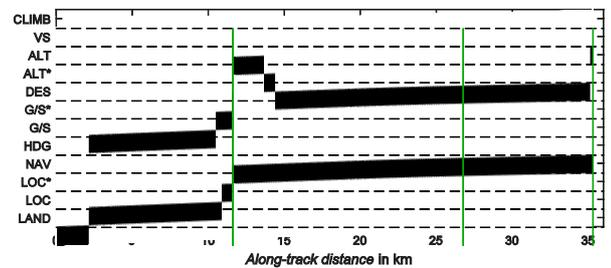
**Figure 4 ILS W180 from 23 July 2015. The top panel shows lateral and vertical flight technical error, the bottom panel indicates autopilot modes active during the approach. Green lines mark the approach waypoints. The dive and drive mode is visible in the vertical modes from kilometer 12 to 15 and in the vertical FTE variation between WFCAF and WB180.**
