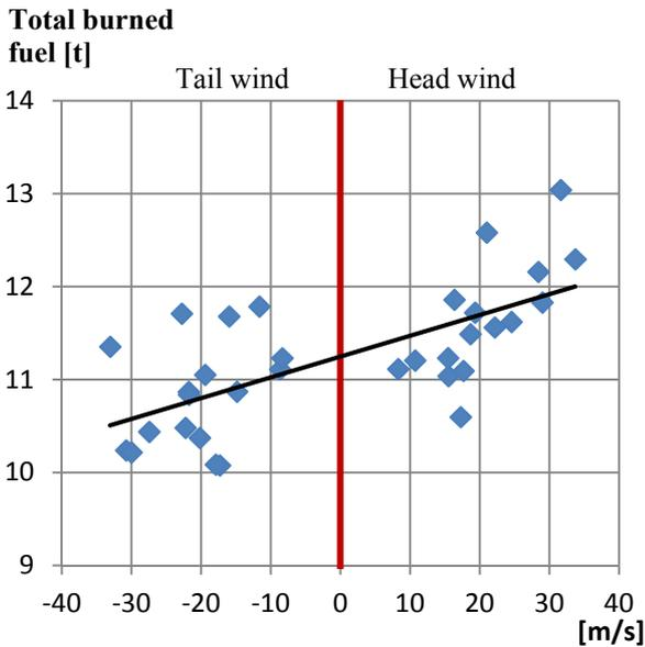
Fig. 8. Total aircraft fuel consumption on certain route depending on axial component of the jet stream
