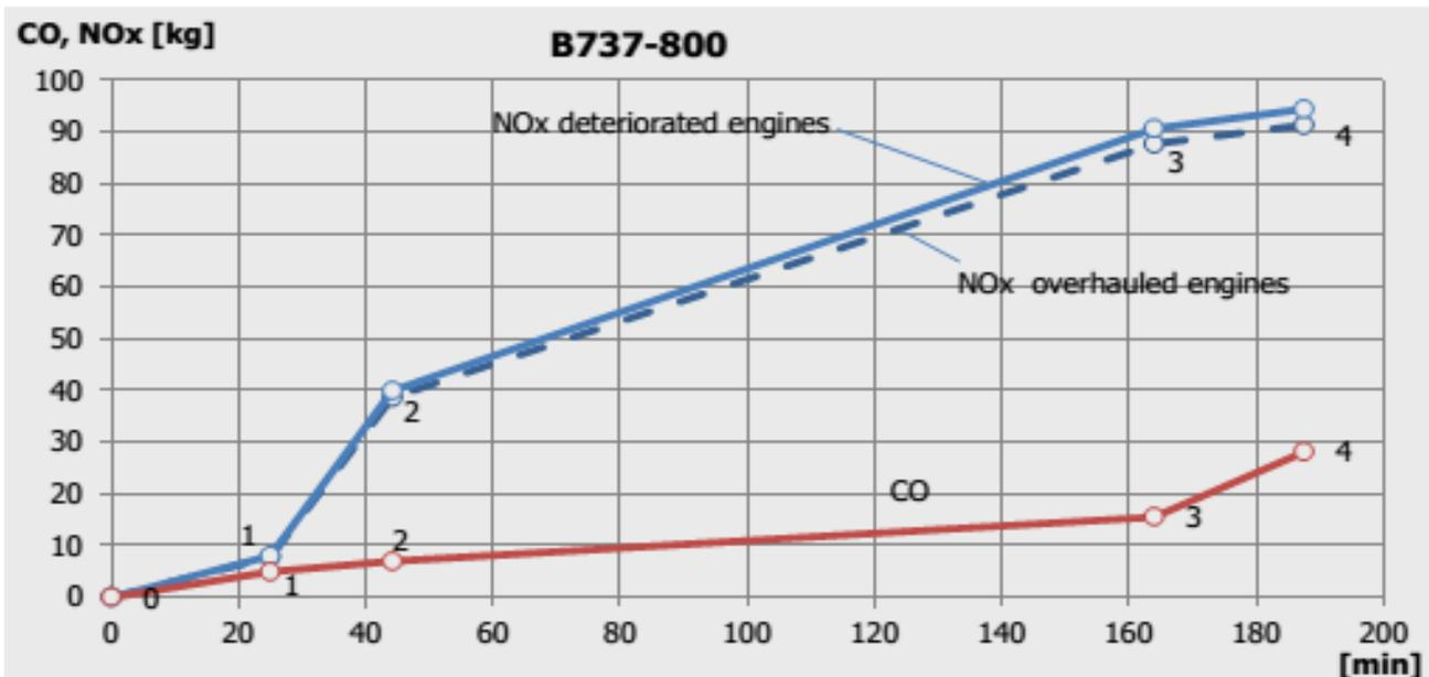
Fig. 3. NOx emission during B737-800 flight while engine deterioration is taken into account. 0-1 Landing and takeoff cycle, 1-2 Climb from 3000 feet to the cruise altitude, 2-3 Cruise, 3-4 Descent to 3,000 feet.
