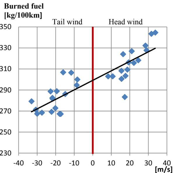
Fig. 7. Aircraft fuel consumption per 100 km depending on axial component of the jet stream
