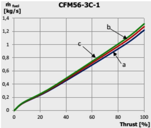
Fig. 1. Fuel consumption of: a-ICAO Aircraft Engine Emissions Databank engine; b, c- test-cell results of overhauled engines.
