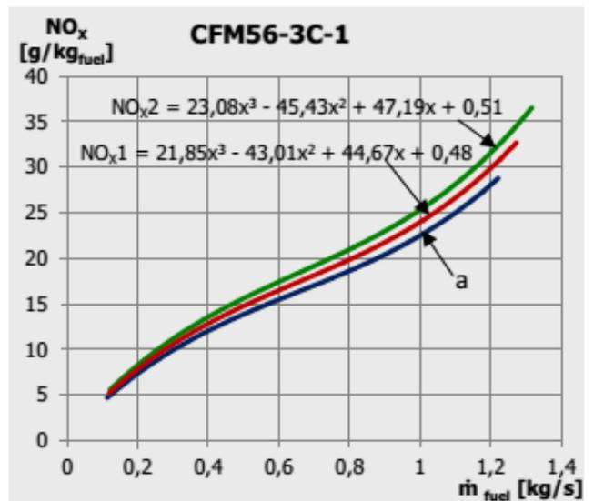
Fig. 2. Dependence of NOx emission from fuel consumption of the installed CFM56-3C-1 engines. Where "a" represents an "ideal" engine.
