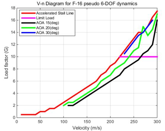
Fig. 3. V-n Diagram for F-16 Pseudo 6-DOF Model
