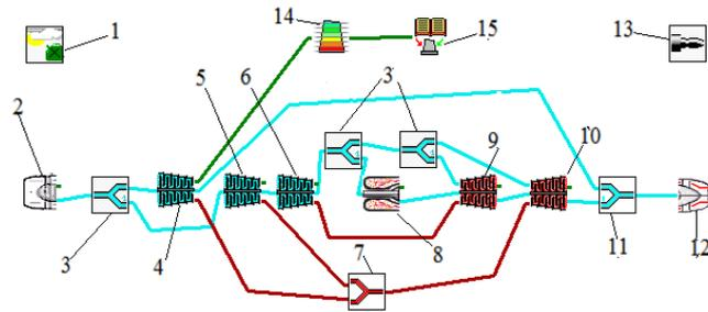
Fig. 1. Topological model PS-90A in ES "AM" for selecting of material, where 1 – SE Initial conditions; 2 – SE Input device; 3 – SE Air bleed; 4 – SE Fan; 5 – SE Booster compressor; 6 – SE High pressure compressor (HPC); 7 – SE Add power; 8 – SE Combustion chamber; 9 – SE High pressure turbine (HPT); 10 – SE Low pressure turbine (LPT); 11 – SE Mixer; 12 – SE Jet nozzle; 13 – SE General results; 14 – SE Strength compressor blades; 15 – SE Material compressor blades.
