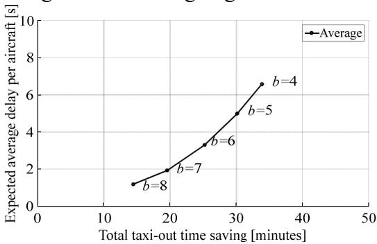
Fig. 4 Relationship between taxi-out time saving and take-off delay using constant buffer method for 6 days average.
