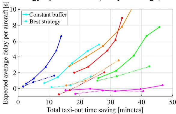
Fig. 8 Relationship between taxi-out time saving and take-off delay using all parameters strategy optimization on each day.
