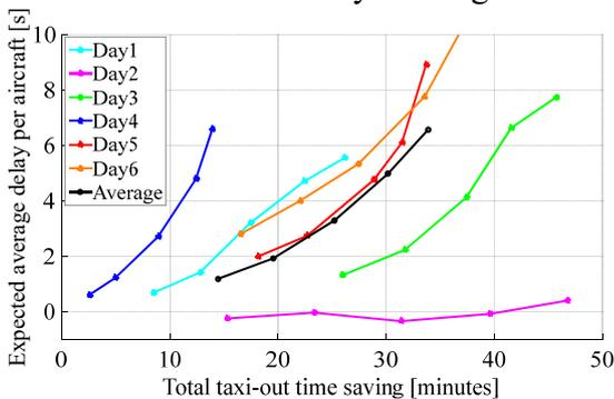
Fig. 5 Relationship between taxi-out time saving and take-off delay using constant buffer method on each day.
