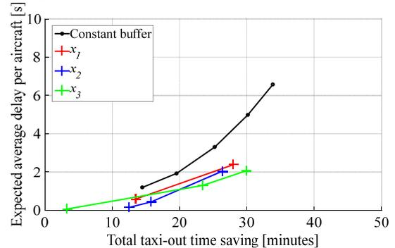
Fig. 6 Relationship between taxi-out time saving and take-off delay using a single parameter strategy optimization. (6 days average)
