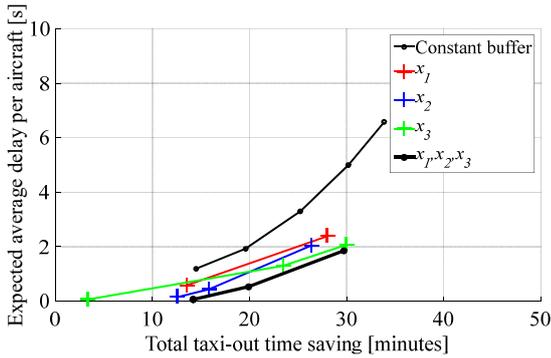
Fig. 7 Relationship between taxi-out time saving and take-off delay using all parameters strategy optimization. (6 days average)
