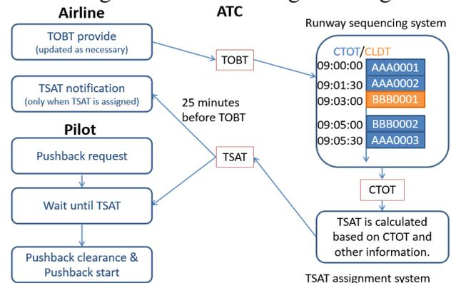
Fig. 2 TSAT operation flow.
