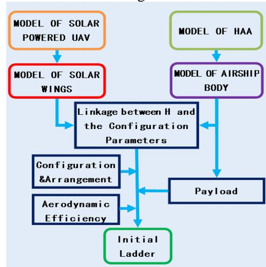
Fig.9 Flow Chart of Concept Design
