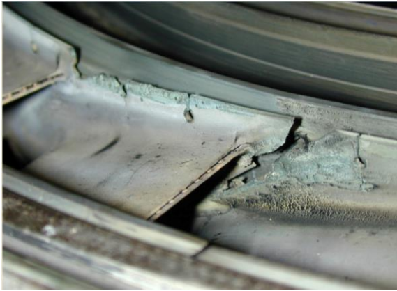
Fig.7. Block of guide vanes of high-temperature film-cooled platforms, formed by a system of single cylindrical channels
